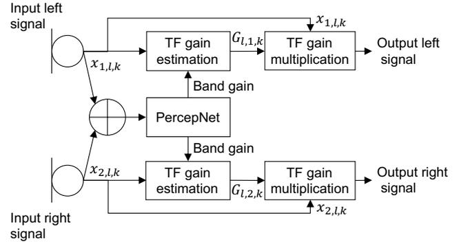
Fig. 2. Block diagram of common-gain method.
