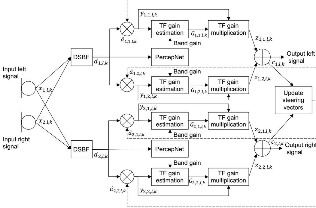
Fig. 3. Block diagram of proposed stereo speech enhancement algorithm.
