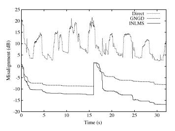
Fig. 4. Normalized misalignment for typical speech input and white Gaussian interference (scenario 2) with an abrupt change in the unknown system  $\mathbf{h}(n)$  at 16 s. The direct algorithm diverges.
