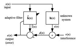
Fig. 1. Block diagram of echo cancellation system.
