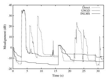
Fig. 5. Normalized misalignment for typical speech input and interference (scenario 3) with an abrupt change in the unknown system  $\mathbf{h}(n)$  at 16 s. Note that the direct method frequently diverges, and the GNGD method diverges less often, but still significantly between 3–4 s, at 6 s, 14 s, and 31 s. All the divergence events are due to double-talk, except at 3–4 s, where only interference is present.
