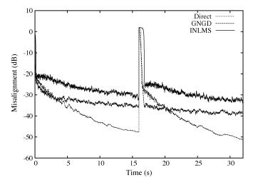
Fig. 3. Normalized misalignment for white Gaussian input and interference (scenario 1) with an abrupt change in the unknown system  $\mathbf{h}(n)$  at 16 s. All algorithms converge.
