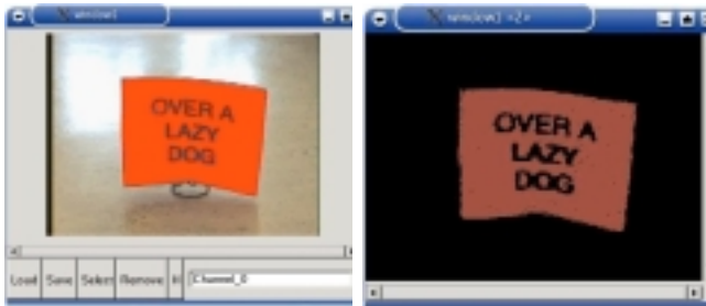
Figure 4. Color training graphical user interface (left) and color perception from the mobile robot (right)
